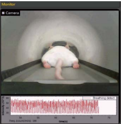
Embedded LED Camera: The camera enables real-time observation of small animals during imaging. Respiratory signals can be detected using camera images and displayed on the interface.
