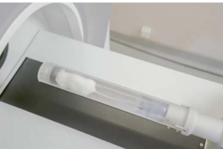
Anti-Escape Cover: This design prevents small animals that are not completely anaesthetized from escaping during the experiment.
